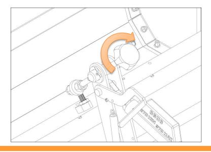
If the machine is being moved between sites it is advised that the brush is taken out of drive. This is done by disconnecting the clutch drives on each wheel (Below left). Always remember to put the clutches back into drive before starting work.
