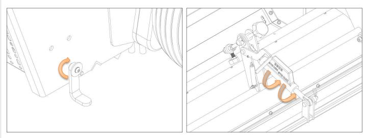
When disconnecting from the vehicle always ensure that the rear stand is down. This keeps the brush bristles clear of the surface to avoid the bristles being deformed.
